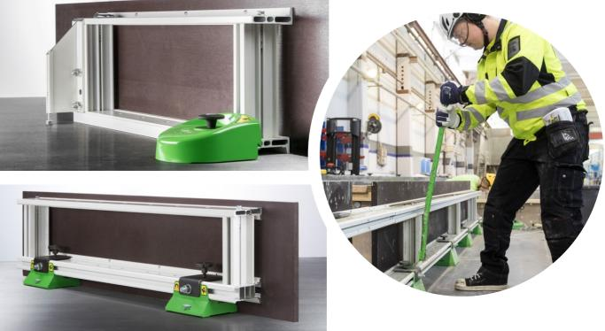
The FaMe Flex system is a costeffective solution for beam and column production when you need flexibility for occasional production. The FaMe Flex system can be used on a hollow-core slab bed, for example.
