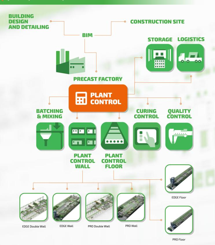
Elematic Plant Control is a production operations management software suite specially designed for precast concrete factories. The system has been developed together with precast producers to make sure that it matches requirements from hollow core to circulation lines.
