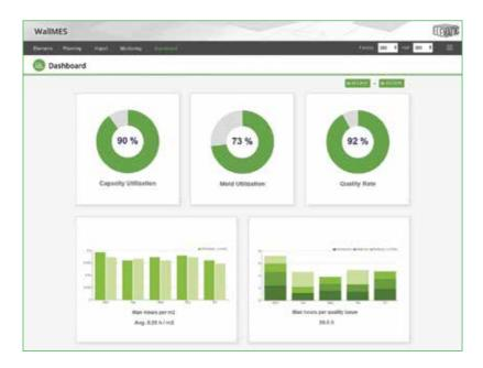
The Elematic Plant Control dashboard uses the data available in the system and shows it in a visual format. It turns data into meaningful factory KPIs.
