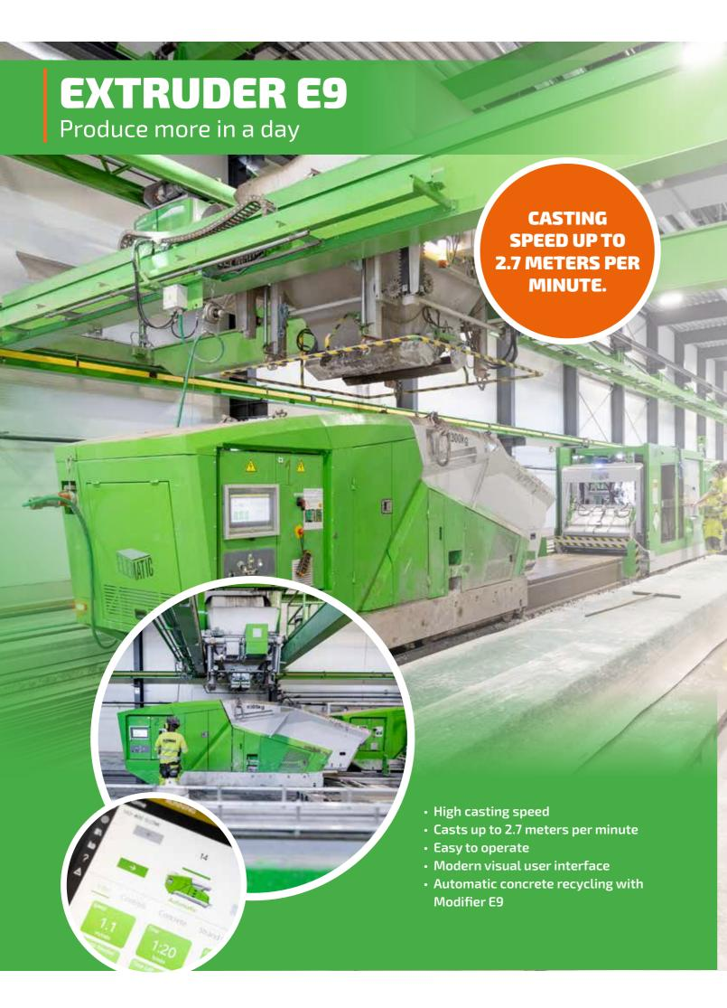
When you need fast slab production, the Extruder E9 suits the requirement perfectly with the industry's highest casting speed of up to 2.7 meters per minute. The high casting speed means it produces 8 to 10 cast beds in the same time that was previously used to produce only 6 cast beds, producing as many as 18 cast beds per day.
