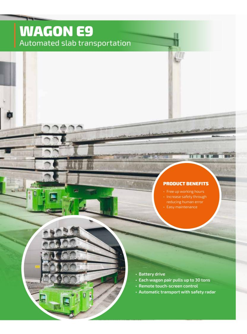
The battery-powered Wagon E9-1200w-b moves slabs quickly from production to storage automatically. The transportation consists of an active and passive wagon with a combined 30-ton capacity.
