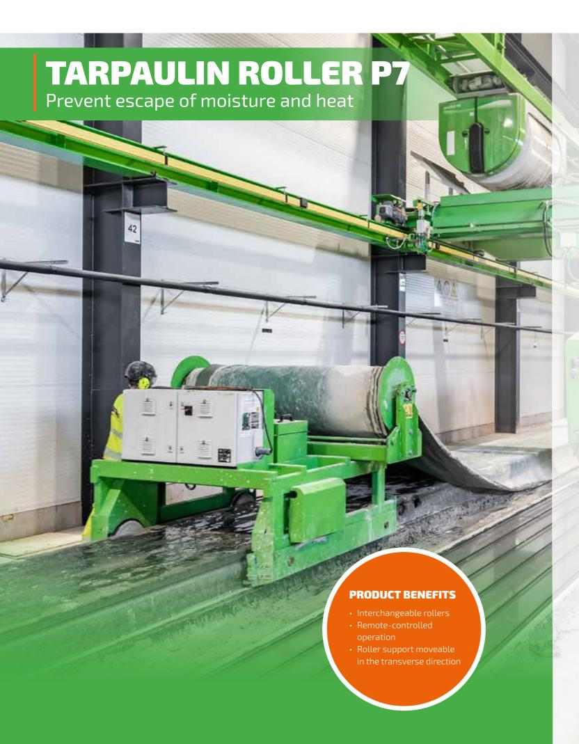
The Elematic Tarpaulin Roller P7-1200t spreads tarpaulins onto slabs and winds them back onto the roller during precast concrete production. Covering the fresh slabs prevents escape of moisture and heat.
