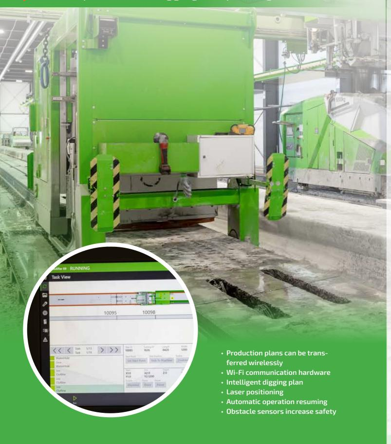
The Modifier E9 is an automatic machine for digging openings and recesses, for example HVAC ducts and plumbing, into fresh hollow core slabs. It also drills water holes and plots cutting lines, openings, and text.
