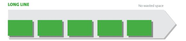
Long line technique in half slab production may supply even 60% better productivity compared to circulation line.
